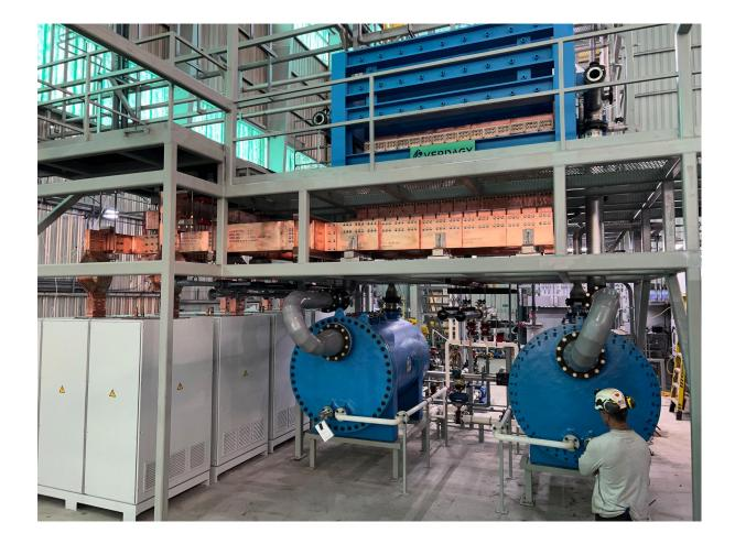
An electrolyzer in Verdagy's pilot plant in Moss Landing, California. The electrolyzer's cells are contained in the blue structure at top, while the cylindrical tanks hold electrolyte. *Source: Verdagy*
