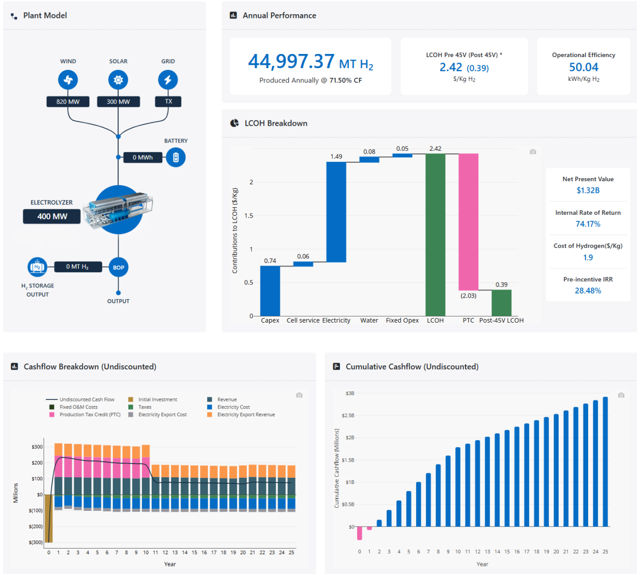
Figure 4: Techno-economics summary for a 400 MW electrolyzer plant in 2030 with Verdagy 1
